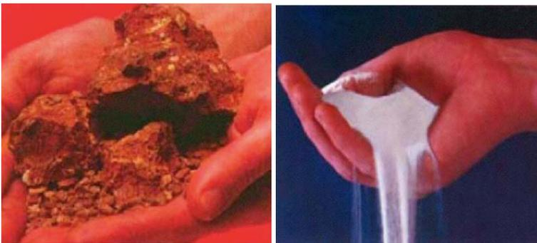
**Figure 9.1:** From bauxite (left) to alumina (right), via the Bayer process (IAI 2006).
