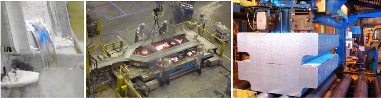
**Figure 10.3:** Illustration of molten aluminium entering the casting process (left); the casting process itself (middle), and the finished ingots as rectangular blocks (right). Pictures are provided by Montembeault (2009).
