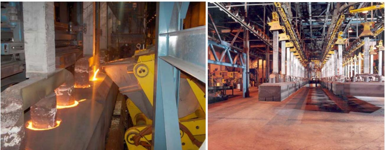
**Figure 10.2:** Attachment of steel rods to anodes (left) and transport of the rodded anodes to the smelter (right). Pictures are provided by Montembeault (2009) and represent pre-bake technology.
