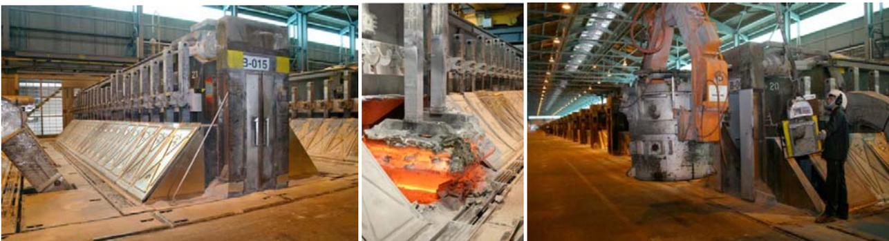
**Figure 10.1:** Illustration of an aluminium pot with multiple anodes at the Alcoa smelter in Deschambault, Quebec (left); change of used anodes (middle), and extraction of molten aluminium from the pot (right). Pictures are provided by Montembeault (2009) and represent pre-bake technology.
